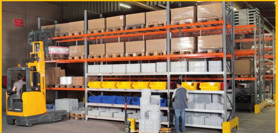
“Hybrid” Epsirack shelving for storing heavy palletised items and for picking.
